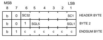
b = Odd Byte Parity Bits. c = Even Column Parity Bits.
